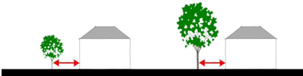
Figure 37: When siting and planting new trees make sure the future size and canopy of the tree is considered in relation to buildings and adequate distance between them
