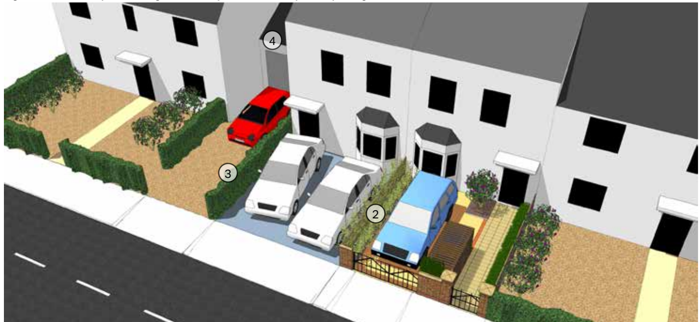
Figure 42: Diagram showing the effect of keeping on plot parking subservient to landscape and property boundary treatment
